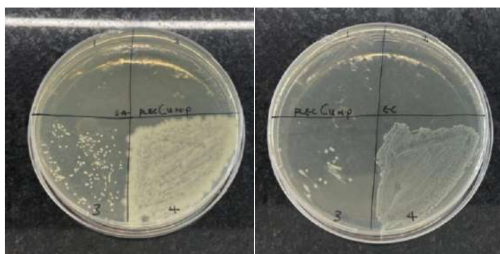
Figure 15: MBC sample plates of copper nanoparticles on E. coli and S. aureus .
