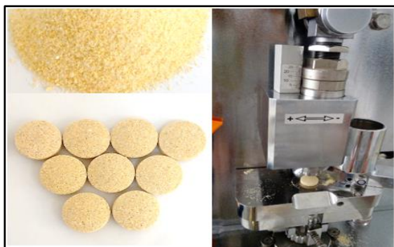
Figure 2: Tableting of granules produced by wet granulation method-1.
