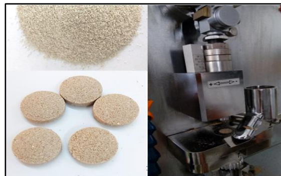
Figure 3: Tableting of granules produced by wet granulation method-2.
