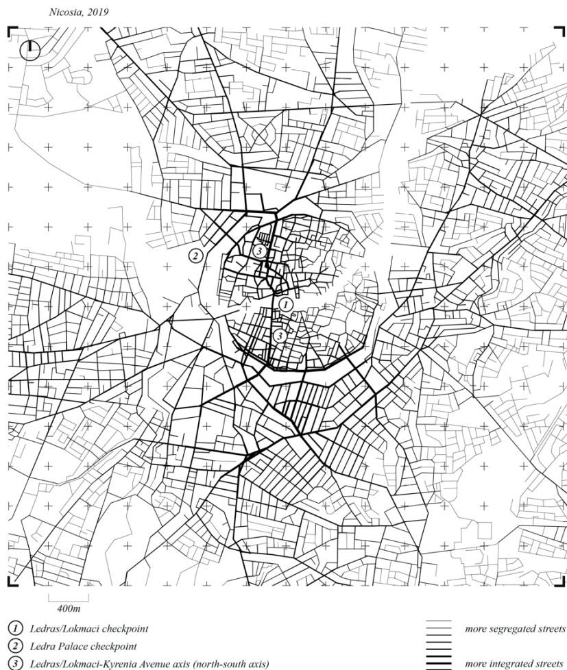
Fig. 2. Axial map of the degree of integration of each road in Space Syntax in 2019 (elaboration of the author)
